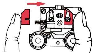
When mounting the motor box, care must be taken not to catch up the connecting cables.
